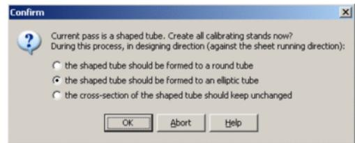
Three methods are available how the defined shaped tube should be formed (against the sheet running direction):
