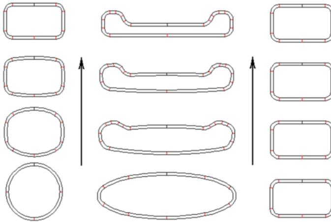
Calibrating shaped tubes from a round tube (left column), from an elliptic tube (center column), and by keeping the cross-section unchanged (right column). The top row shows the final product and the bottom row the cross-section in the welding station. The arrows point in tube running direction.
