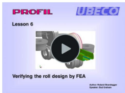
You learn how to verify the roll design by [FEA - Finite Element Analysis](#). The FEA system LS-Dyna is a suitable instrument to check if the designed rolls are able to produce the desired profile with the requested allowances. The handling procedure is shown for the example bumper project.
